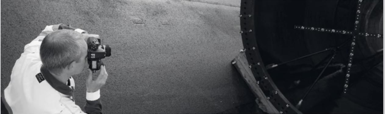
Blades, towers, and nacelles are all constructions where size and accessibility can hinder efficient quality control. Optical 3D coordinate measuring is possible in harsh environments using GOM's optical metrology solutions. The measuring systems define the exact 3D (XYZ) positions of markers and visible features for inspection, analysis and quality control.
